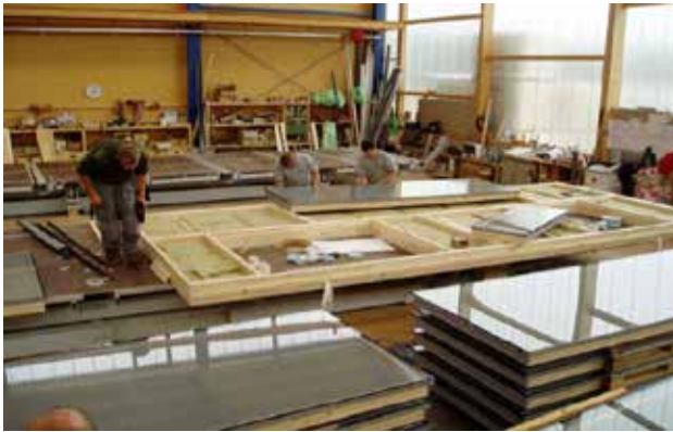
Figure 5 Preparation of SCIMFS units and attaching them to the existing wall [10]
