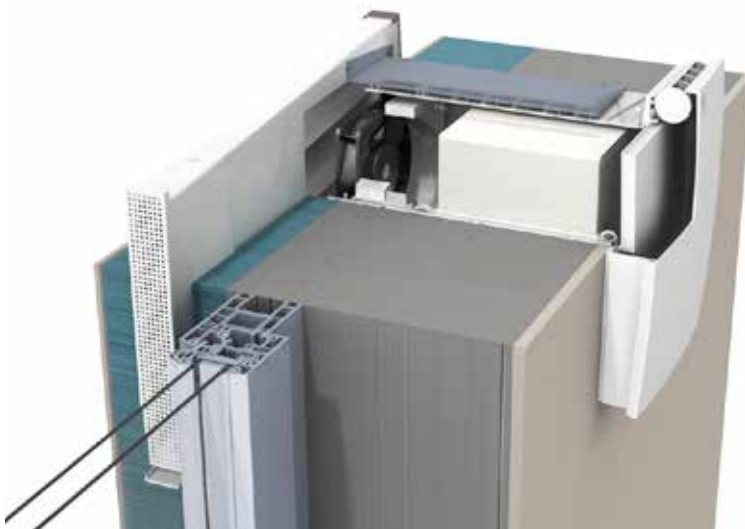
Figure 04, Decentralized ventilation unit inside the wall
