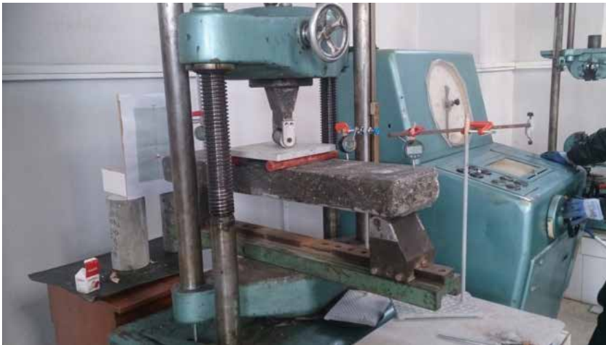
Figure 6. View of the tension by bending test
