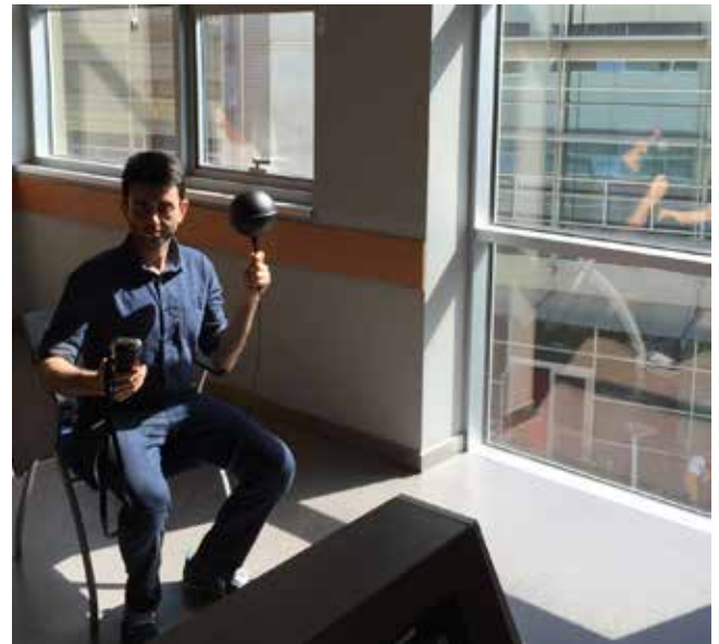
Figure 7 Mean radiant temperature measurement on the surface of person
