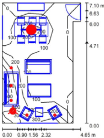
Figure 10: Isolux curves related to lighting design for Suggestion 1
