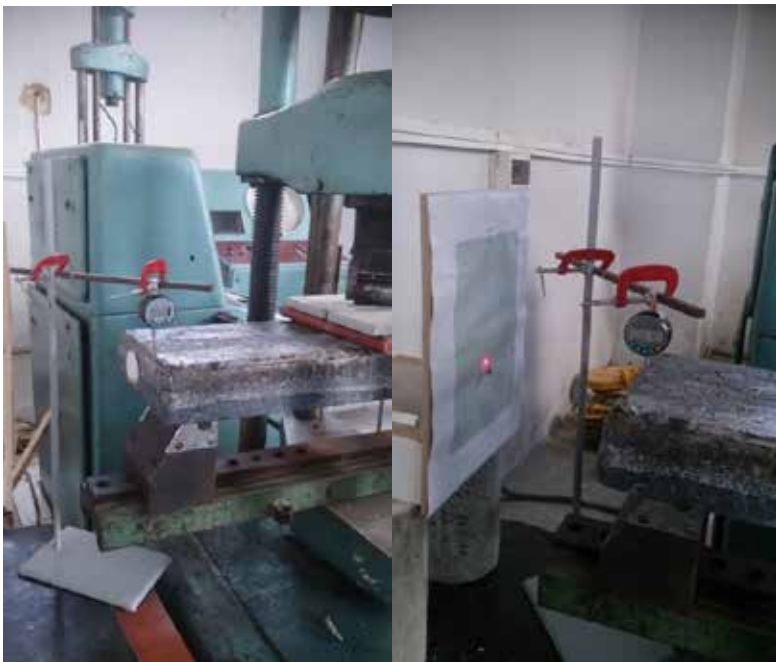
Figure 7. Rotation angle measurement of the tension by bending test
